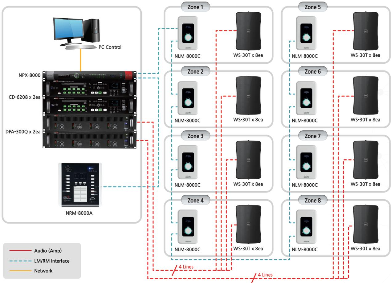
The NPX system is a distributed control audio matrix device that outputs audio sources to a desired area through various source devices, SD cards, etc. With NRM-8000A (4 units can be linked), announcement can be broadcast by selecting the desired area, and the matrix, volume, and DSP can be easily set up with MP-8000(integration control program) and mobile application.
